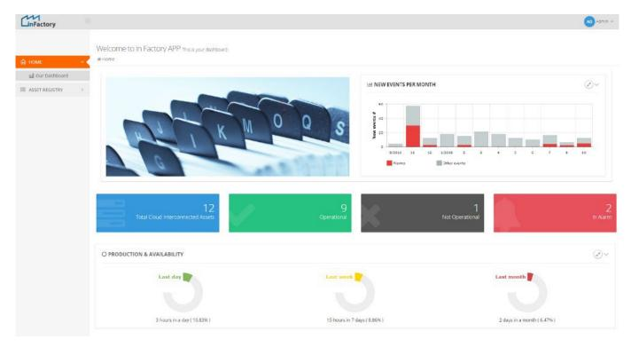
With the purchase of inFactory and the successful interconnection of at least one machine, the customer will have access to a dedicated web portal from which it is possible to monitor the collected telemetry. Furthermore, access to the visualization software of the production plan set for a specific machine directly via the HMI interface installed on the machine operator panel will be given.
