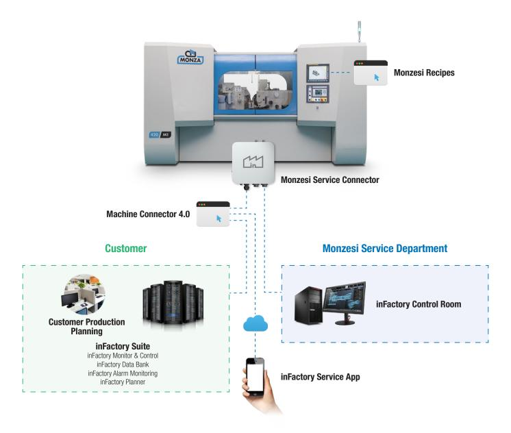
The main modules of the inFactory architecture therefore concern both the data collection policies on site as well as their processing on cloud systems, and therefore the distribution of information to the machinery.
