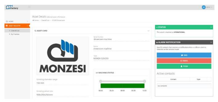
The software module offers the possibility of issuing bulletins and reports on the alarms identified and processed by the machinery to operators/managers through digital communications (e.g. SMS, e-mail, PUSH app).
